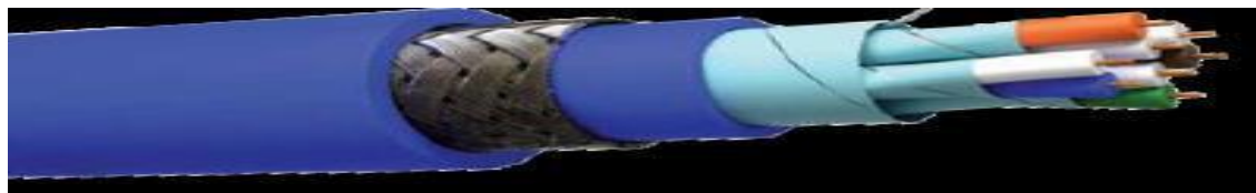
F/FTP LAN Marin cable 4x2x23AWG - cat .6 - LSZH shf2
